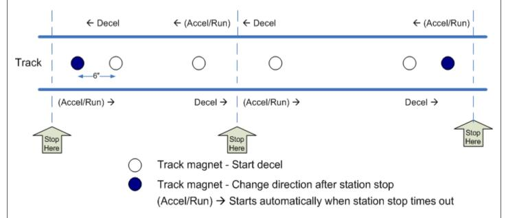
Automated station stops are initiated by a track magnet placed ahead of the station. The magnet initiates deceleration to a stop. You can make as many stops as you like, one magnet per station. When running in both directions, two magnets per station are required, one for each direction. Place the magnets such that the loco stops at the same location when running from either direction. The magnet in front of the locomotive when leaving the station will be ignored.
