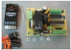
What you get: RailBoss Plus board, and 4 R/C cables. The DSM2 compatible receiver (upper left) is not supplied.
