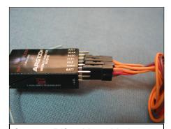
Connect R/C cables with the orange (data) wire towards the top of the Rx. The BATT slot remains open, unless being used for binding.
