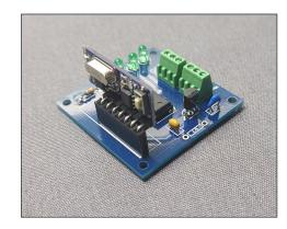
Transmitter buttons 1 - 4 control outputs D3/B,D2A,D1/D, and D0/C respectively.
