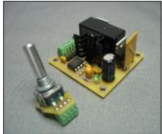
Basic Critter Control board and rotary speed switch module with built-in push button.
