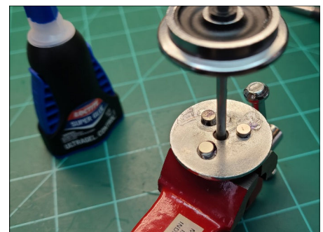
Three magnets were too close together on this 1.2" dia. Wheel. I had to use two.
