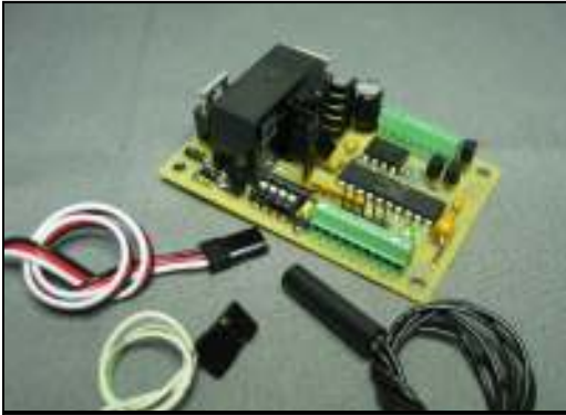
This is what you get: The RailBoss R/C Enhanced board, 3-wire Rx cable, 1-wire Rx cable, and a reed switch.
