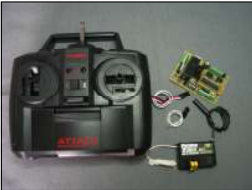
To complete the system, you must also supply a suitable hobby transmitter and receiver. Shown here is a typical 75 MHZ AM 2-Channel stick radio and receiver. (Shown here: Futaba Attack 2DR)
