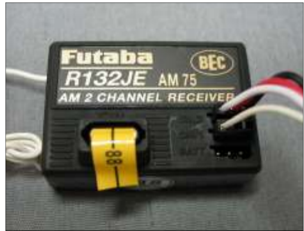
A typical 2-channel receiver with 3 connectors: CH2 (3 wire cable for power and speed), CH1 (1 wire cable for direction), Batt (not used). Note: The order of these plugs and the orientation of the cables will differ between manufacturers.
