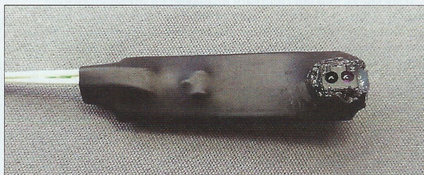
5. To help protect them from dirt, each sensor and its little board are wrapped in heat-shrink tubing.
