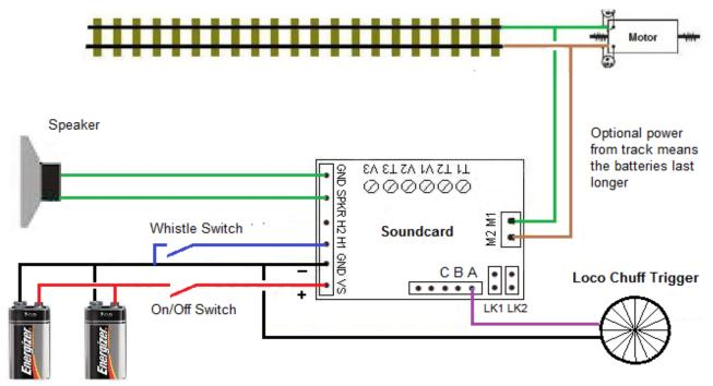
Use one small 9v battery for moderate volumes Use two small 9v batteries or one larger one for maximum volumes The DC track voltage can vary from zero to a maximum of 24 volts. Controllers should be linear not pulse width modulated. On DCC systems you must connect the soundcard to the DC output to the motor, not to the AC voltage from the track.
