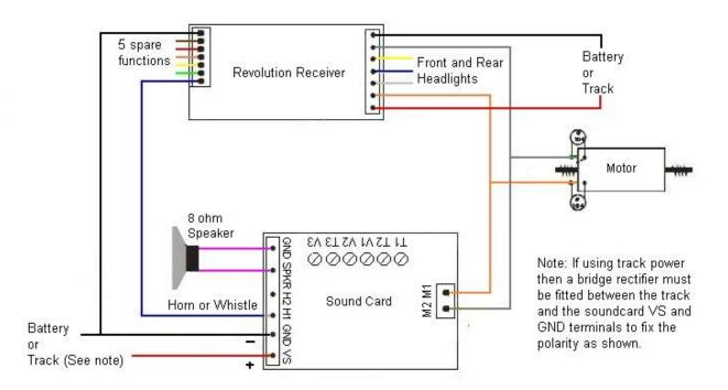
The diagram below shows how the soundcard can be connected to the Train Engineer Revolution from Aristocraft for both battery and track power supply. If using track power then you will need to purchase a bridge rectifier from your local consumer electronics store. Connect it between the track and the soundcard with the positive going to the VS terminal and the negative to the GND terminal.
