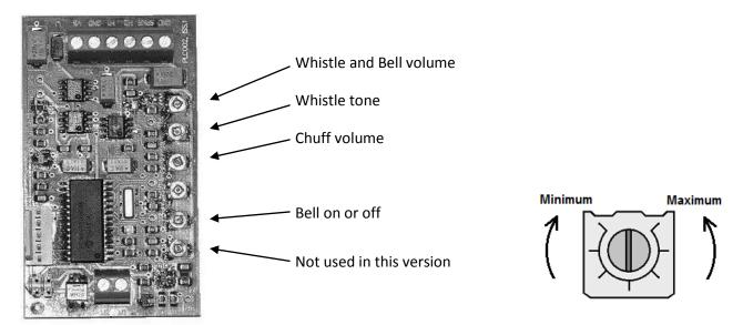
Note that each trimport rotates between the minimum and maximum positions shown above. Turn anti-clockwise to increase the setting and clockwise to decrease.
