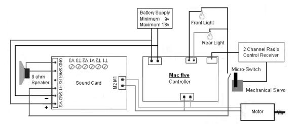
The Brian Jones Mac Five uses one channel for loco speed and direction but has no accessory channel. The second channel can drive a separate mechanical servo and micro switch to operate the whistle. The wiring diagram is shown above.
