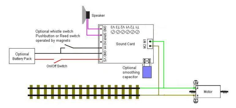
The sound card is designed for use on track powered railways where the DC voltage varies from zero to a maximum voltage of between 7.2 and 24 volts. Controllers should be linear not pulse width modulated. On DCC systems you must connect the soundcard to the DC output to the motor, not to the AC voltage from the track.
