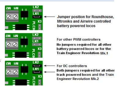
For all other controllers which output plain DC, both jumpers must remain fitted to LK1 and LK2 as shown. These include track powered locos and the Crest Train Engineer Revolution Mk.2 from Aristocraft.
