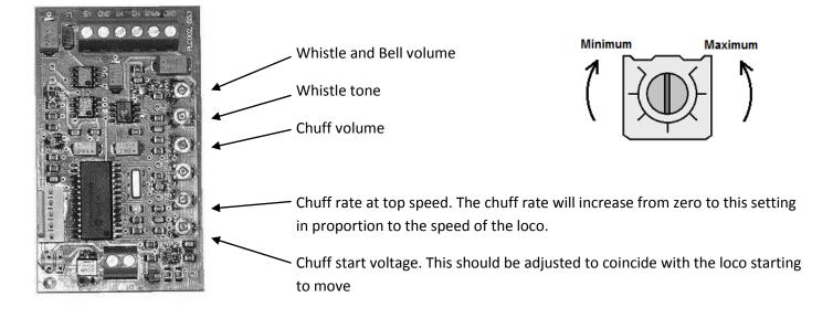
Note that each trimport rotates between the minimum and maximum positions shown above. Turn anti-clockwise to increase the setting and clockwise to decrease.
