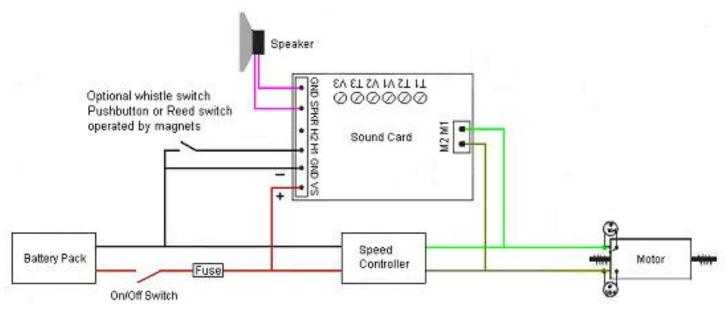
Again, the whistle can be operated by means of a switch or pushbutton mounted on the loco, by means of a reed switch operated by trackside magnets or by modifying a wireless door chime or garage door opener. It sounds when the switch is closed and stops when the switch is opened. The whistle is shown as a negative (ground) input connected to terminal H1.
