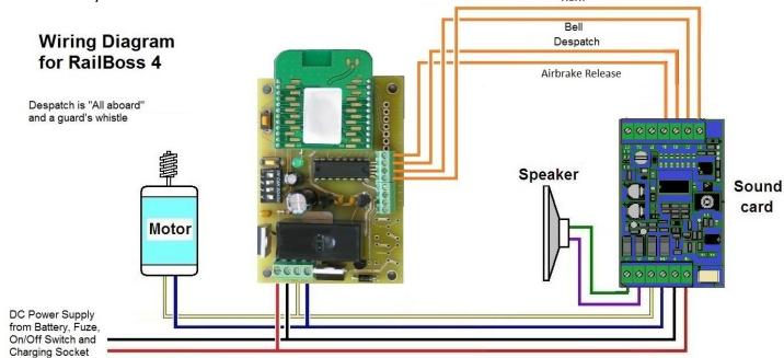
The RailBoss 4 can trigger four sound functions. The fifth and sixth soundcard triggers, the turbocharger and engine start/stop, therefore cannot be radio controlled and will need to be switched on, if required, by the IR remote control or be set to sound automatically.
