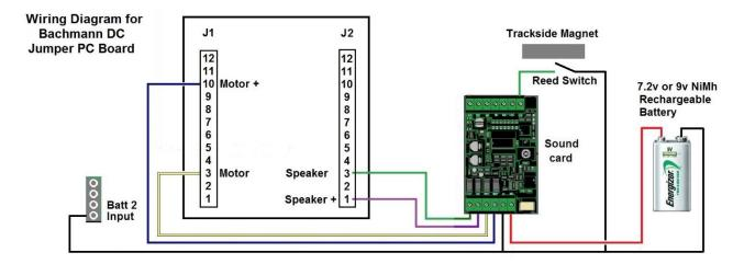
On DCC track powered railways in locomotives using a basic decoder, the wiring is a little different:
