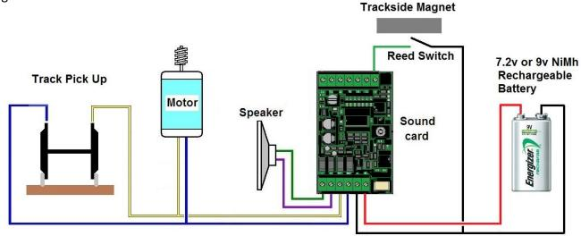
The wiring diagram below shows the connections for the DC jumper board in a Bachmann locomotive.
