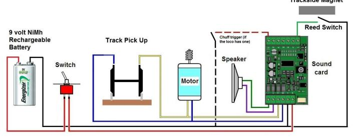
When the track voltage is below nine volts it is insufficient to power the soundcard. Therefore a nine volt PP3 battery is used to drive the soundcard and produce sound when the loco is static or moving slowly.
