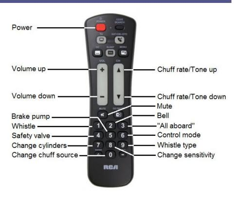
Note that the buttons on the remote control auto-repeat if held down. If you want a single event to occur, like turning on the safety valve, then press the safety valve and release it immediately. If you want to make a large change in volume or tone then you can hold the button down to avoid the need to press the button repeatedly.
