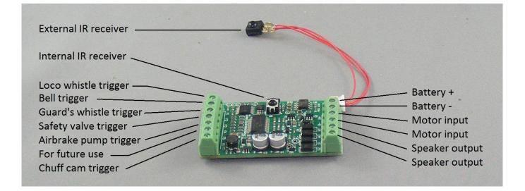
The soundcard generates synthesised sound which is adjustable to reproduce the sounds of most steam locos and railmotors. The terminal connections on the right are necessary for the soundcard to generate a chuff which varies with the loco speed and load. The terminal connections on the left trigger the various sounds where the locomotive controller has the appropriate outputs available.
