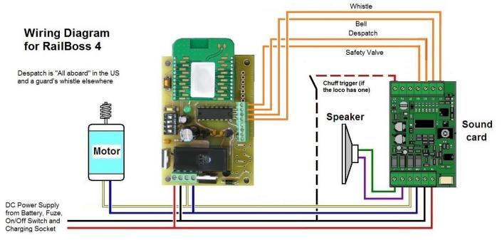
The RailBoss 4 can trigger four sound functions.
