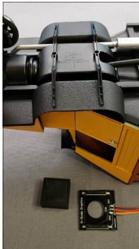
3D printed spacer block and reed switch PCB
