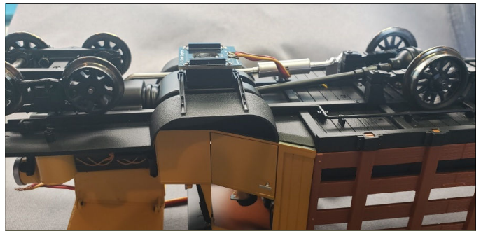
Mounted reed switch assembly
