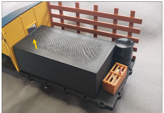
New 3D printed box covers it all. IR sensor peeks out of the box.
