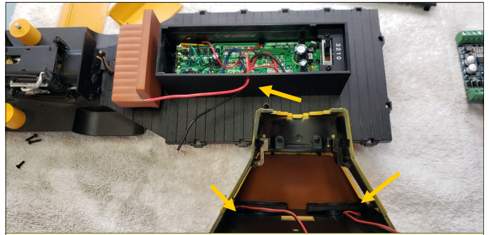
Track power wires routed out of factory electronics box. Two small speakers were mounted in roof of the cab.
