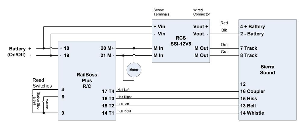
Due to the design of the Sierra Sound Board, the RailBoss motor output is not directly compatible with the Sierra inputs. An RCS SSI-12V5 board must be used to provide power and motor isolation to the Sierra.
