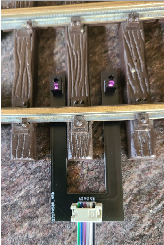
Speed sensor. The camera sees the IR light (pink) that we can't see with the naked eye.
