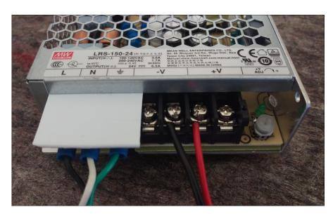
Crimp some spade connectors on the wire ends for a nice neat connection. The AC input terminals on your power supply may be exposed, so you may want to insert a piece of styrene over them for added safety.
