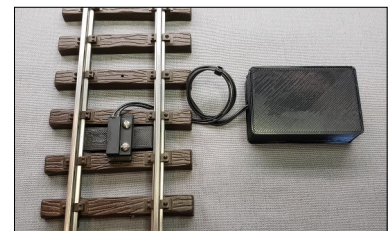
Wireless Reed Switch talks to receiver in TrackSide
